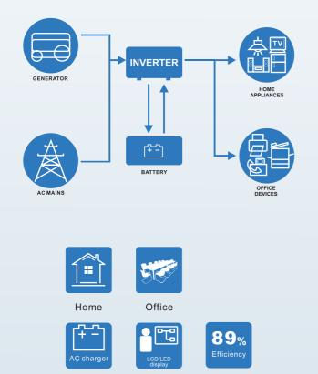
The HD500-2000VA series inverter/ charger system converts DC power to AC power with amazing transfer efficiency. With the continuous output and compact design,the HD is excellent for home and office environment.Appliances such as TVs,stereos, desktop or laptop computers and others can be connected to HD for the uninterruptible power.
